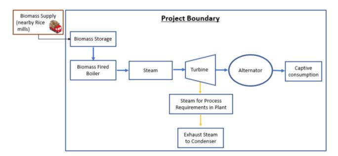
In line with this methodology, the project boundary encompasses the industrial facility of the company, equipment installed for the operation of cogeneration plant, the biomass storage facility, the facility (paper mill) consuming the energy (electrical and thermal) generated by the project activity plant; Plant would use biomass as a renewable fuel of the boiler. Quantity of the biomass
